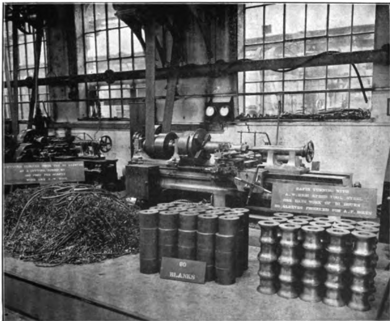
B. Turning sleeves for armour-plate bolts in 12-inch high-speed lathe. 60 bolts produced per day, of 10 hours. Cutting speed, 160 feet per minute; depth of cut, \frac{1}{4} ; feed, \frac{1}{16} ; weight removed from each blank, 36 lbs.; total weight removed, 2160 lbs. (Sir W. G. Armstrong, Whitworth & Co., Ltd., Manchester.)
